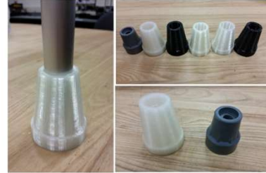
Figure 3. (Left) A 3D printed crutch tip installed onto a crutch. (Top Right) Different iterations of 3D printed material to test crutch tips. (Bottom Right) A 3D printed crutch tip in comparison to original crutch tip.
